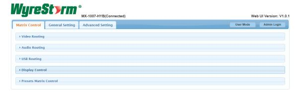
• In User mode, users can also click "Admin Login" on the upper right corner, then input the password enter Matrix Control, General Setting and Advanced Setting pages. The default password is "admin". When login the admin mode first time, users also need to change login password first. The operations are same with logging through the home page.
