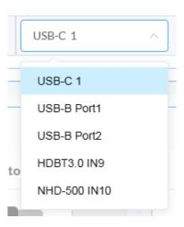
For example, when selecting USB-B Port1, all USB devices the matrix connected and the remote receivers connected are connected with USB-B Port 1.
